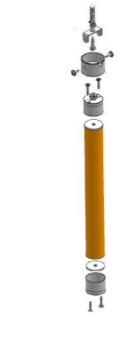
Ceiling installation “I”Shape installation
