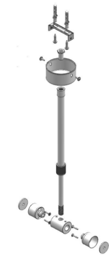
Pendant pole “—” Shape installation “Ω” type installation
